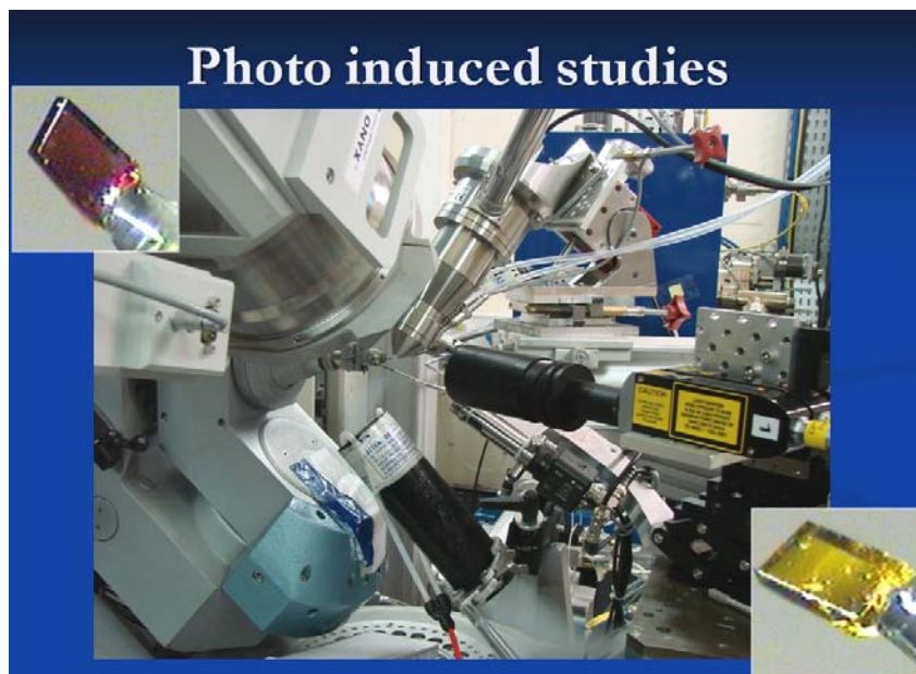
Figure 4. Example of an in-situ experiment carried out on the KM6 diffractometer
