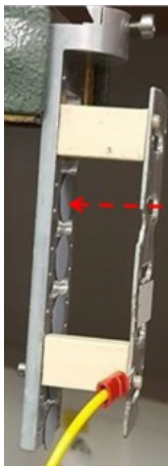
Figure 5: Total Electron Yield device.
