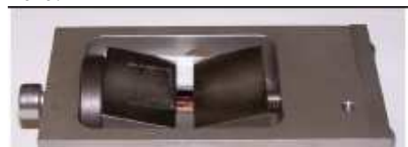
Figure 1: copper bi-crystal in the compression machine. The loading electric motor on the left side is unmounted here.
