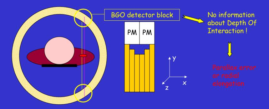
DOI measurement with the design of LXe  $\mu$ -PET
