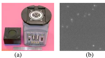
Figure 1: (a) A photograph of the newly developed EMCCD camera, and (b) an image showing sensitivity of the camera to individual 122 keV \gamma -ray photons from a ^{57}\text{Co} source.
