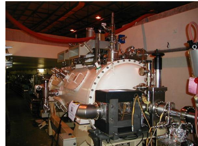
SOLEIL Voltage: up to 5 MV TTC Power: up to 400 kW
