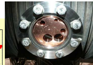
window with new HOM shielding
