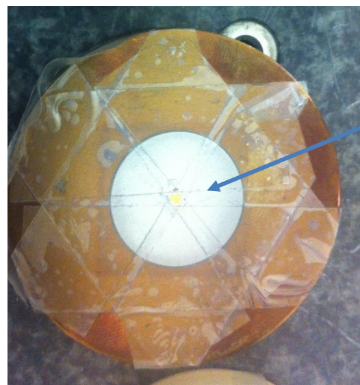
LiNbO 3 crystal (glued on the backside of the anvil)
