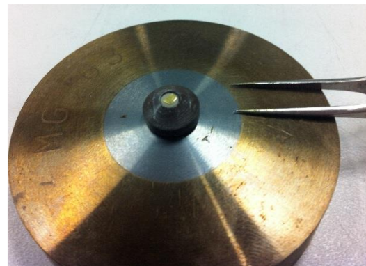
Cell assembly (gold foil to improve MHz wave transmission)
