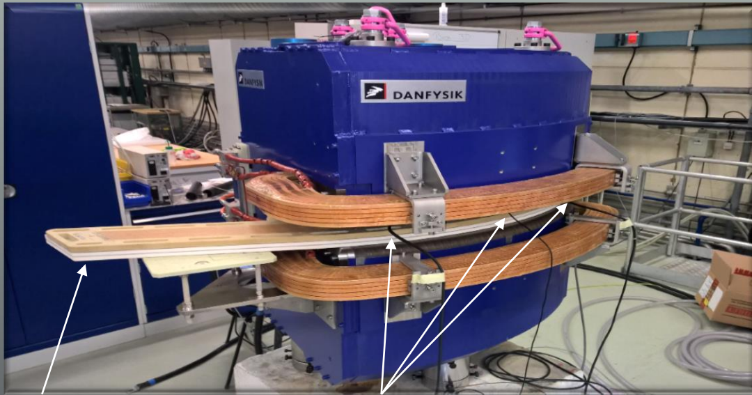
curved fluxmeter for the integral field (both dynamic and DC-equivalent at the end of each staircase plateau) 3 × Projekt Elektronik AS-NTM-2 Hall probes moved sequentially to 12 on-axis positions
