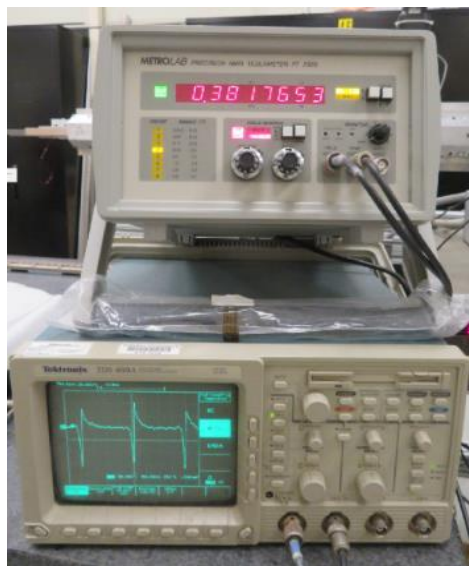
Hall Sensor Voltage calibration against NMR_Probe Metrolab PT 2025 03/14/19 Annex, CHESS
