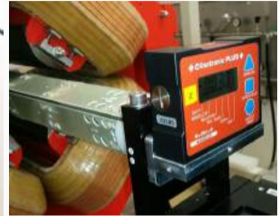
Clinometer support for calibration of coil angle at acquisition start
