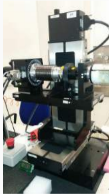
Stage A (left), Stage B (right) Bellow to transmit rotary motion Slip rings Cylindrical bearings
