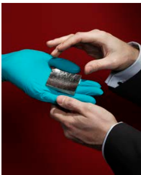
Figure 1: HAPG as the decisive material of a wavelength dispersive element in laboratory spectrometers for reasonable measurement times.
