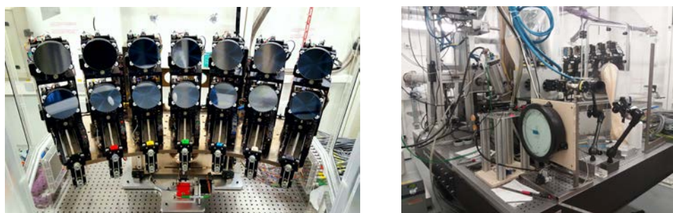
Figure 1: 14-crystal Crystal Analyzer Spectrometer (left), in operation with hydrothermal cell (right)
