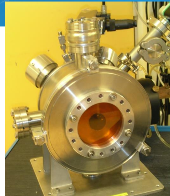
Induction furnace 3000 °C
