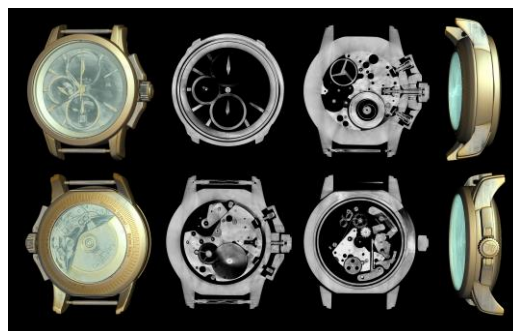
Figure 1: Synchrotron CT scan of a high-grade mechanical wrist watch (18.5 \mu m/voxel).
